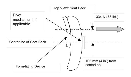
Figure 16g - Off-center Backrest Durability Loading - Right
