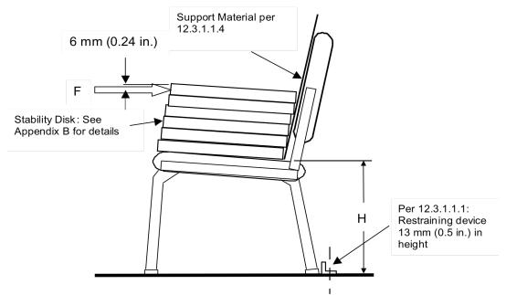
Figure 12a - Rear Stability Test for Type III Chairs
