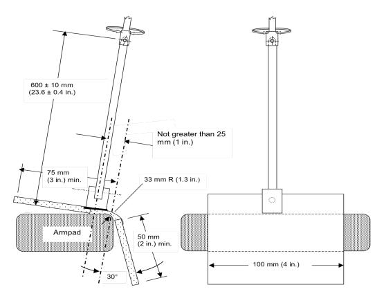
Figure 21a - Arm Loading Device
