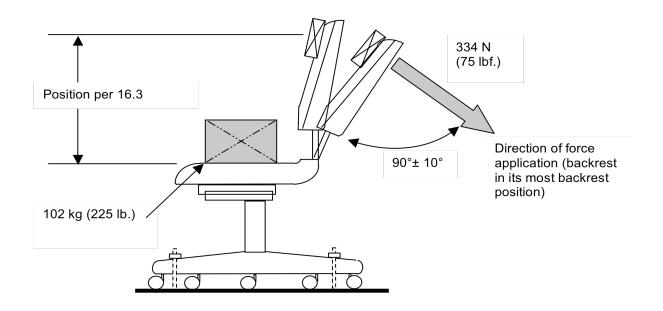
Figure 16e - Force Application for All Other Backrests Backrest Durability Test - Cyclic - Type II and III
