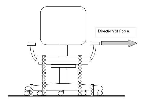
Figure 14 - Arm Strength Test - Horizontal - Static
