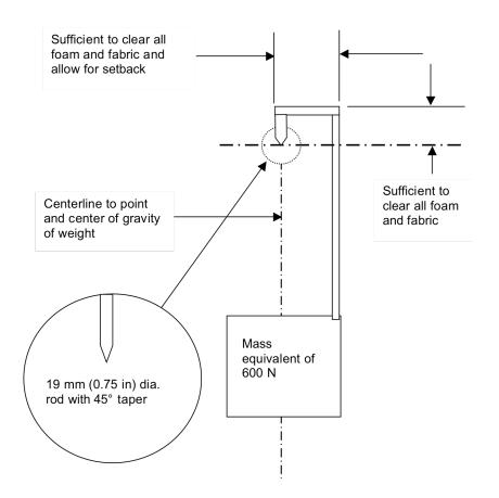
Figure 12g - Front Stability Loading Fixture
