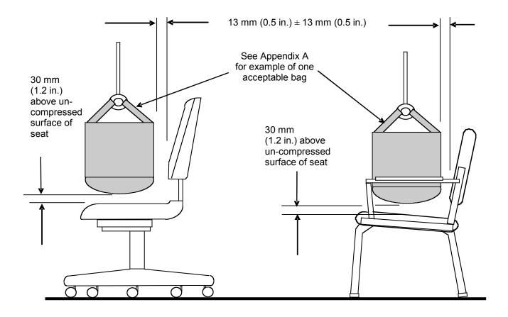
Figure 11a - Seating Durability Test - Cyclic
