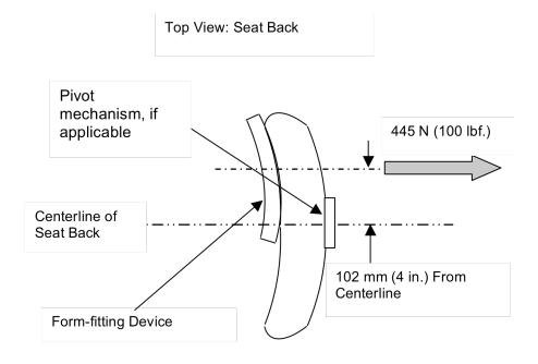
Figure 15g - Off-center Backrest Durability Loading - Right
