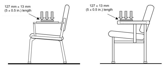
Figure 13a - Arm Strength Test - Vertical - Static
