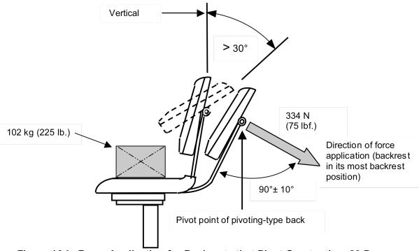
Figure 16d - Force Application for Backrests that Pivot Greater than 30 Degrees
