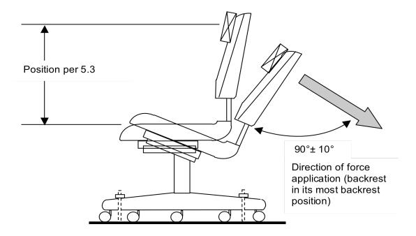
Figure 5e - Force Application for All Other Backrests Backrest Strength Test - Static - Type I
