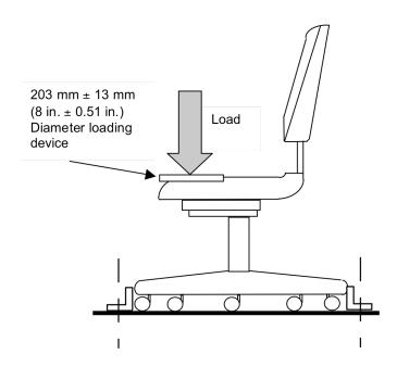
Figure 11b - Front Corner Load-Ease Test - Cyclic - Off-center
