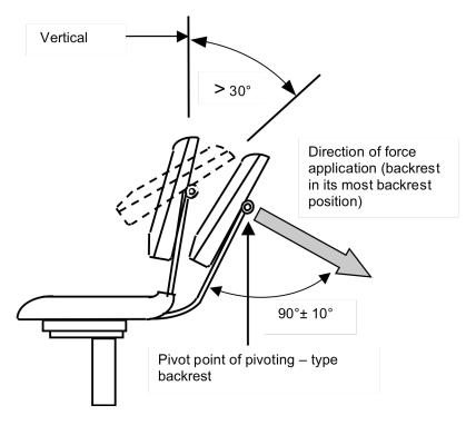
Figure 6d - Force Application for Backrests that Pivot Greater than 30°
