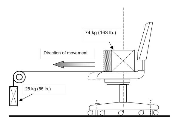
Figure 22 - Out Stop Test for Chairs with Manually Adjustable Seat Depth
