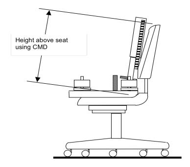
Figure 15a - Test Height Determination Backrest Durability Test - Type I
