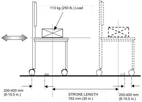
Figure 17e - Machine Schematic for Chairs with Legs
