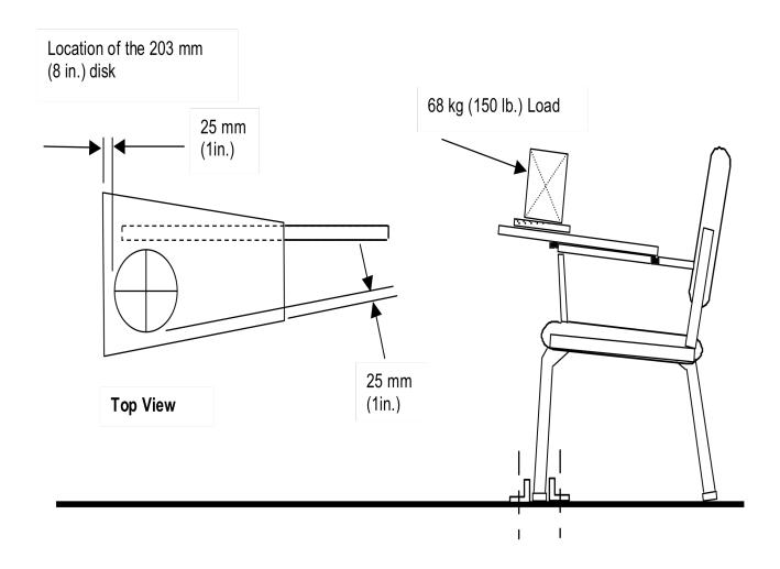
Figure 23 - Tablet Arm Chair Static Load Test
