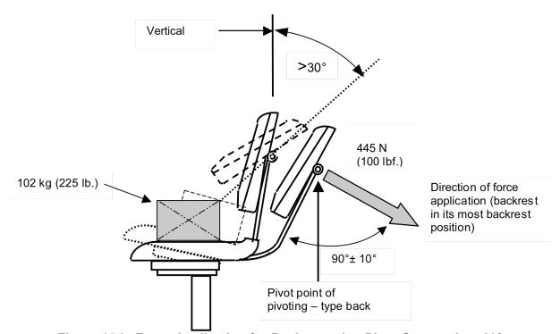
Figure 15d - Force Application for Backrests that Pivot Greater than 30°
