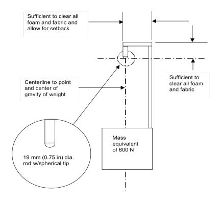
Figure 12d - Front Stability Loading Fixture
