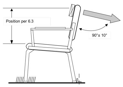
Figure 6e Force Application for All Other Backrests Backrest Strength Test - Static - Types II and III
