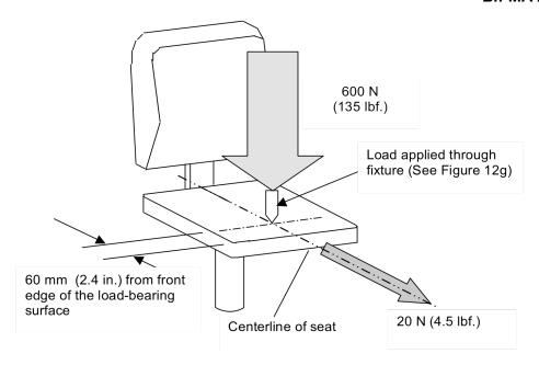
Figure 12f - Front Stability Test
