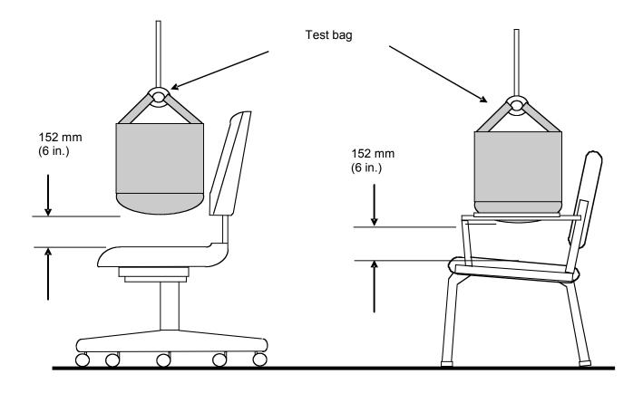
Figure 8 - Drop Test - Dynamic
