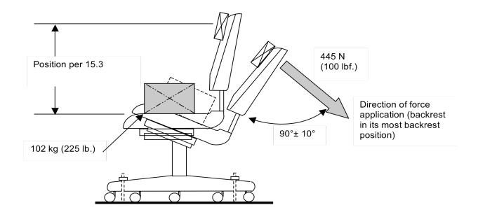
Figure 15e - Force Application for All Other Backrests Backrest Durability Test - Cyclic
