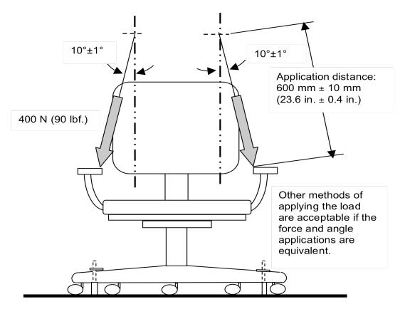
Figure 21b - Arm Durability Test - Cyclic
