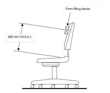
Figure 15b - Positioning of Form-Fitting Device for Backrests Higher than 452 mm (17.8 in.) Backrest Durability Test - Type I
