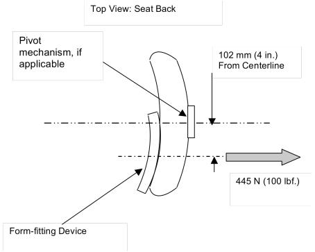
Figure 15f - Off-center Backrest Durability Loading - Left
