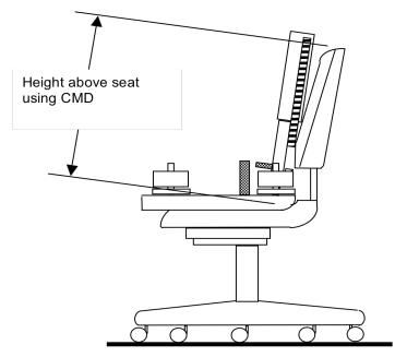
Figure 16a - Test Height Determination Backrest Durability Test - Type II and III
