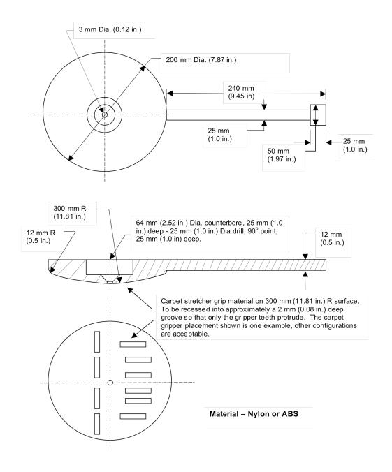
Figure 12e - Front Stability Loading Disk
