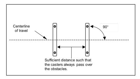
Figure 17d - Obstacle Layout for Chairs with Legs
