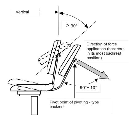
Figure 5d - Force Application for Backrests that Pivot Greater than 30° Backrest Strength Test - Static - Type I
