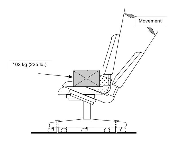
Figure 10 - Tilt Mechanism Test - Cyclic
