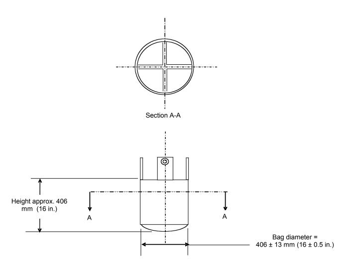
Bag to contain a sufficient quantity of media to bring the bag to the specified load. Media may be shot, slugs, punches, sand, etc. Media may be contained within smaller individual bags/compartments. Media may not be a singular solid material (e.g. single steel or concrete mass).
