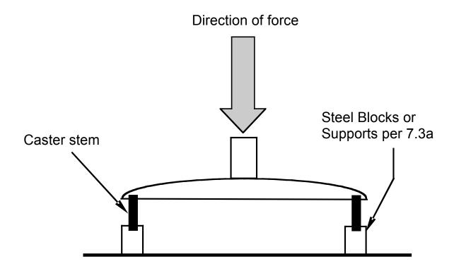
Figure 7 - Base Test - Static
