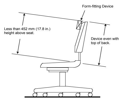
Figure 16c - Positioning of Form-Fitting Device for Backrests Lower than 452 mm (17.8 in.) Backrest Durability Test - Type II and III
