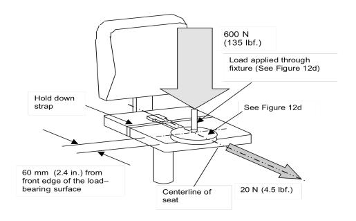
Figure 12c - Front Stability Test
