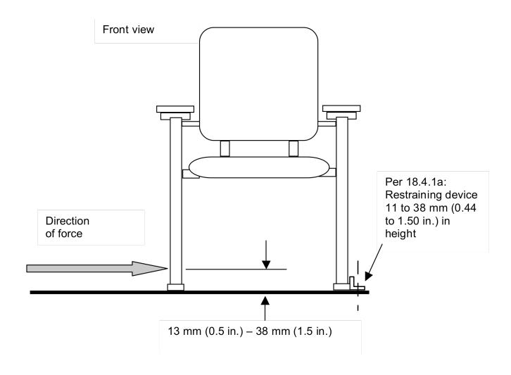
Figure 18b - Leg Strength Test - Side Application
