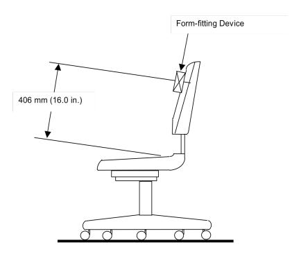
Figure 16b - Positioning of Form-Fitting Device for Backrests Higher than 452 mm (17.8 in.) Backrest Durability Test - Type II and III
