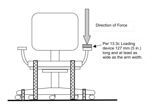
Figure 13b - Arm Strength Test - Vertical - Static
