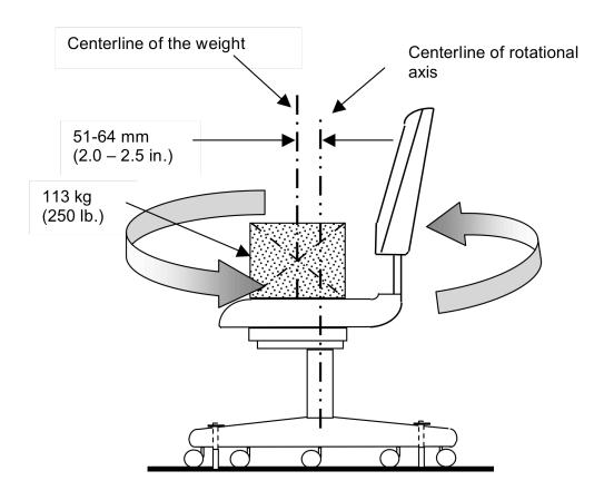
Figure 9 - Swivel Test - Cyclic
