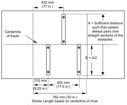
Figure 17b - Obstacle Layout for Pedestal Base Chairs
