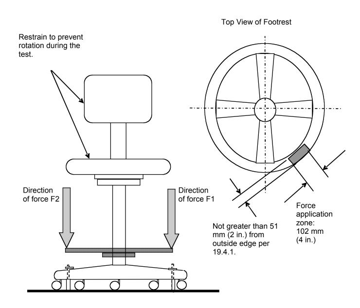
Figure 19 - Footrest Static Load Test - Vertical
