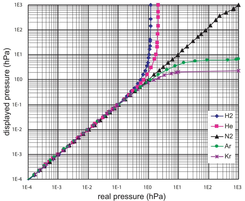
Fig. 11: Measurement curve 200 (Pirani) using the following correction factors
