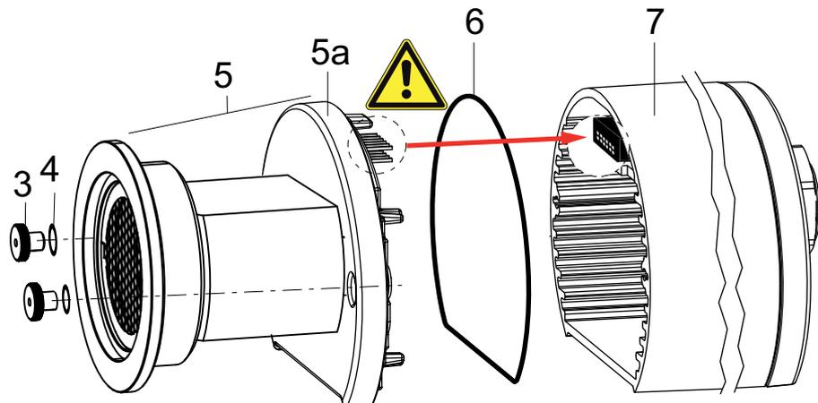
Fig. 8: Replacing the sensor assembly
