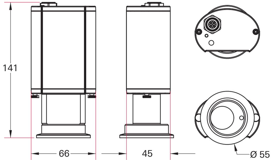
Fig. 9: HPT 200, DN 40 ISO-KF
