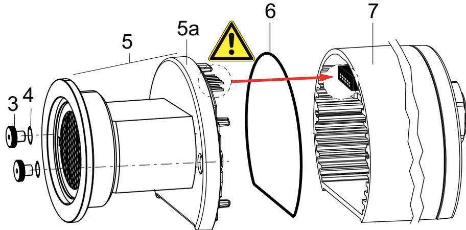
Fig. 6: Replacing the sensor assembly
