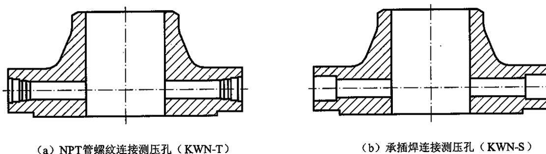
(a) NPT管螺纹连接测压孔 (KWN-T)
