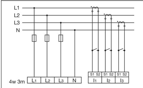
Measurement via 3 voltage transformers in a three-phase 4-conductor network with asymmetric loading.
