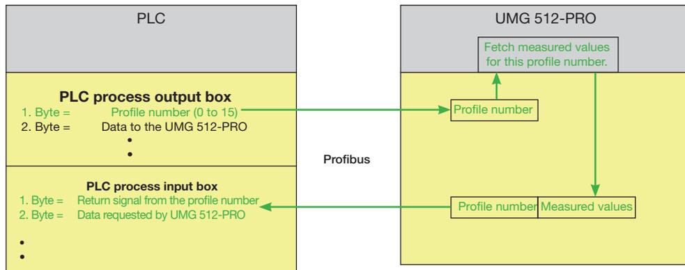
Fig. Block diagram for data exchange between PLC and UMG 512-PRO.
