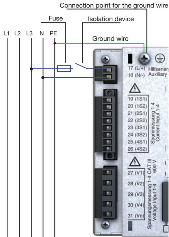
Fig. Example connection for the supply voltage
