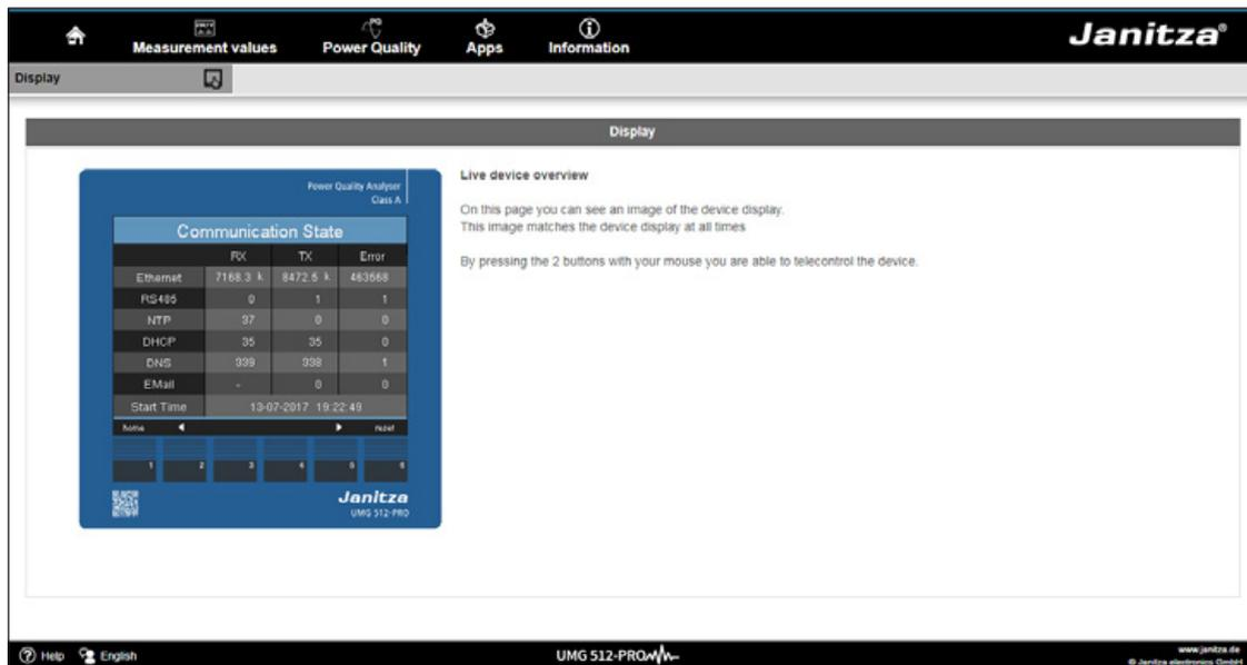
Fig. Operating the UMG 512-PRO via the device homepage
