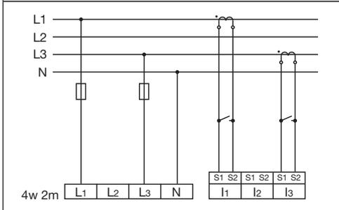
Measurement via 2 voltage transformers in a three-phase 4-conductor network with asymmetric loading.
