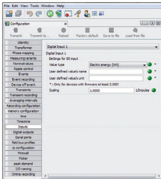
Fig. Configuring the UMG 512-PRO inputs via GridVis®.
