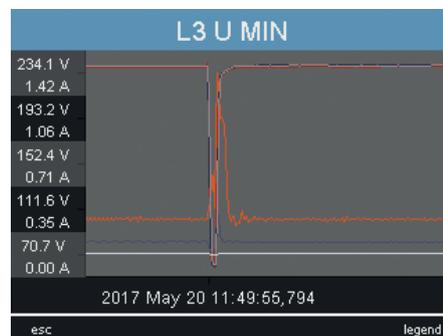
Fig. Illustration of the half wave effective values for an event
