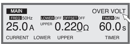
In such a case, set the test current value and upper reference value so that the setting falls within the operation range (b).
