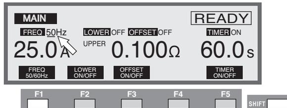
You can set the test frequency using the SHIFT + F1 key combination (pressing the F1 key while holding down the SHIFT key.) Pressing SHIFT + F1 toggles between 50 Hz and 60 Hz settings.
