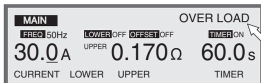
For example, when the test current of TOS6200 is 30 A, if the load resistance (including the resistance of the DUT, the test leads, and any other associated items) from the perspective of the output terminals exceeds  $0.166 \Omega (\cong 150/30^2)$ , the output power exceeds 150 VA, causing an overload. This disables testing.
