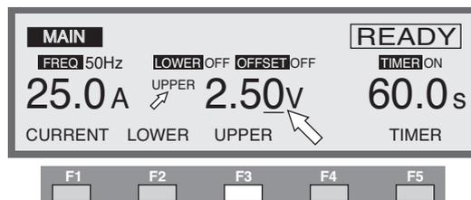
1. Press the F3 (UPPER) key if the upper reference value is not displayed on the LCD. (You can also use the ▲▼◀▶ keys to move the cursor when the upper reference value is displayed.)
