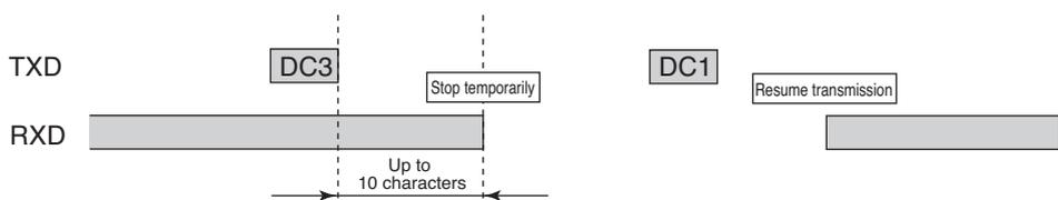
The RS-232C terminal must temporarily stop transmission within 10 characters after receiving a DC3.
