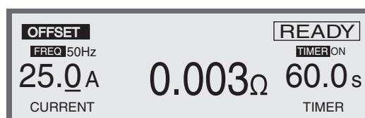
4. If necessary, set test current, test frequency, and timer values.
