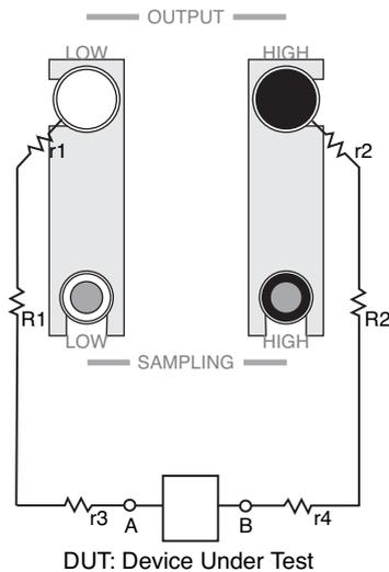
Install the short-circuit bars between the OUTPUT and SAMPLING terminals and connect the leads as shown in Fig. 2-5. The tester measures the total resistance value of contact resistance  $r1$  to  $r4$ , resistance components  $R1$  and  $R2$  of the leads, and the resistance between A and B.
