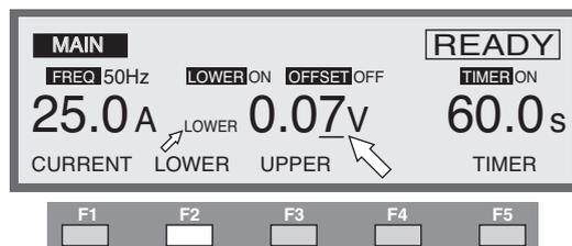
1. Press the F2 (LOWER) key if the lower reference value is not displayed on the LCD. (You can also use the  $\blacktriangle$   $\blacktriangledown$   $\blacktriangleleft$   $\blacktriangleright$  keys to move the cursor when the lower reference value is displayed.)
