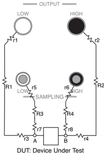
Remove the short-circuit bars connecting the OUTPUT and SAMPLING terminals and connect the leads as shown in Fig. 2-4.
