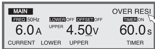
In such a case, set the test current value and upper reference value so that the setting falls within the operation range ㉠. If a resistance value is set to the upper reference value, OVER RESI check is not made.
