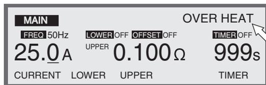
Internal temperatures will fall to normal levels in approximately 10 minutes if no parts are failure. Once temperatures return to normal, press the STOP switch to cancel overheating protection.
