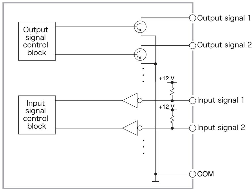
Fig. 5-4 Internal Configuration of the SIGNAL I/O Connector
