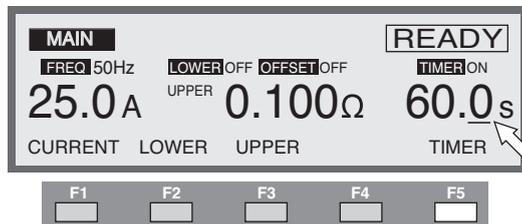
1. Press the F5 (TIMER) key to move the cursor if the cursor is not below the timer (you can also move the cursor using the ▲▼◀▶ keys).
