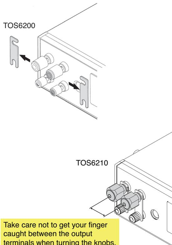
2. Connect the current output line on the crimp terminal side of the test lead (black or white) to the LOW side of the OUTPUT terminals; connect the voltage measurement line on the banana plug side to the LOW side of the SAMPLING terminals. Check that the connections are secure.
