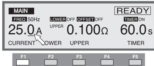
1. Press the F1 (CURRENT) key to move the cursor to the test current value if it is not already there (you can also move the cursor using the  $\blacktriangle$   $\blacktriangledown$   $\blacktriangleleft$   $\blacktriangleright$  keys).
