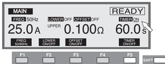
Pressing the SHIFT and F5 keys together allows you to toggle the timer function ON/OFF. Pressing SHIFT + F5 toggles between ON and OFF.
