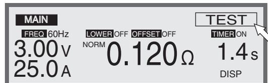
The time indicated after start of the test differs with the timer function set to ON or OFF.
