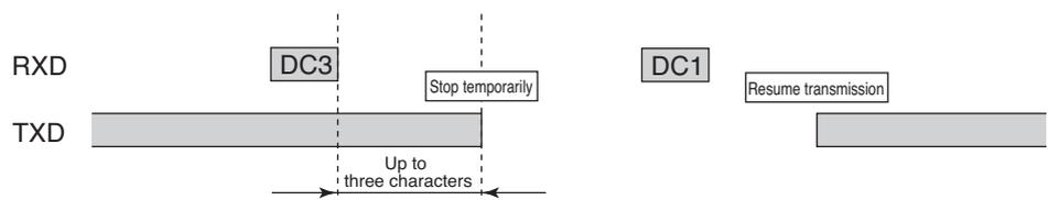
The tester temporarily stops transmission within three characters after receiving a DC3.
