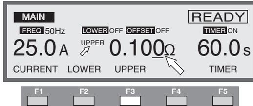
1. Press the F3 (UPPER) key if the upper reference value is not displayed on the LCD. (You can also use the  $\blacktriangle$  $\blacktriangledown$  $\blacktriangleleft$  $\blacktriangleright$  keys to move the cursor when the upper reference value is displayed.)
