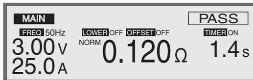
When a PASS judgment is returned for the measured value, "PASS" appears in the upper right part of the LCD, the PASS LED indicator lights, and the buzzer sounds. The PASS judgment is generally displayed for about 0.2 seconds (default value). You can set the PASS judgment display time in the range 0.2 s to 10.0 s or to HOLD. For information on altering this setting, see 4.4, "System Setup."
