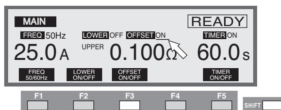
Pressing the SHIFT and F3 keys together allows you to toggle the offset canceling function ON/OFF. Pressing the SHIFT + F3 toggles between ON and OFF.
