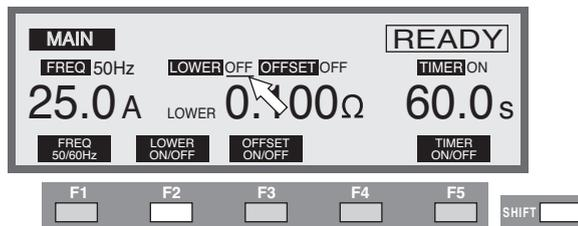
Pressing the SHIFT and F2 keys together allows you to toggle the lower limit judgment function ON/OFF. Pressing SHIFT + F2 toggles between ON and OFF.
