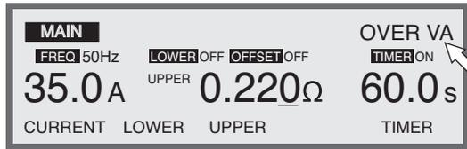
In such a case, set the test current value and upper reference value so that the setting falls within the operation range ㉟. If the offset canceling function is ON, the upper reference value inclusive of the offset value is checked.
