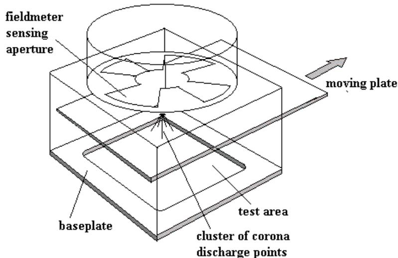
Figure 3.7 Arrangement for measurement of corona charge decay
