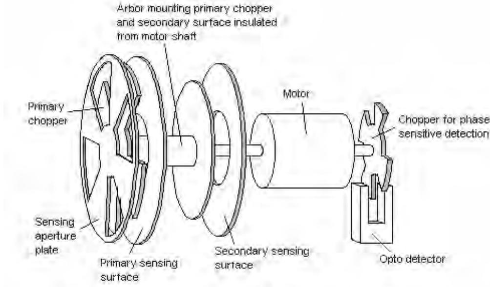
Figure 3.5: 'Field mill' fieldmeter with no earthing of the rotating chopper
