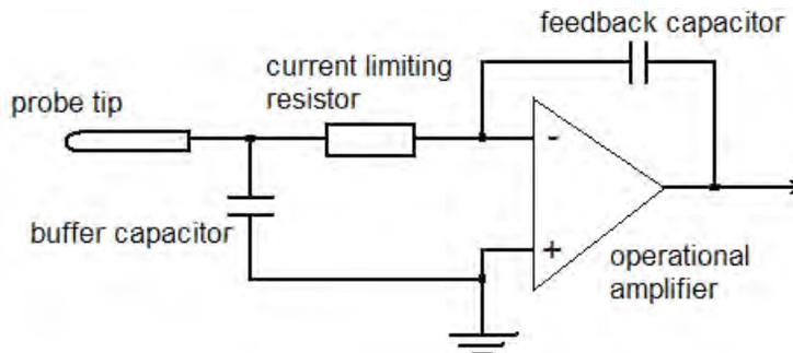
Figure 3.18: Example of buffer capacitor with virtual earth charge measurement amplifier
