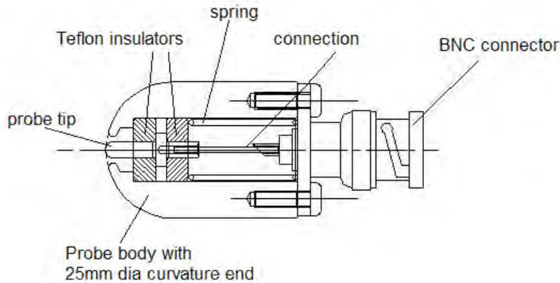
Figure 3.17: Example of shielded probe
