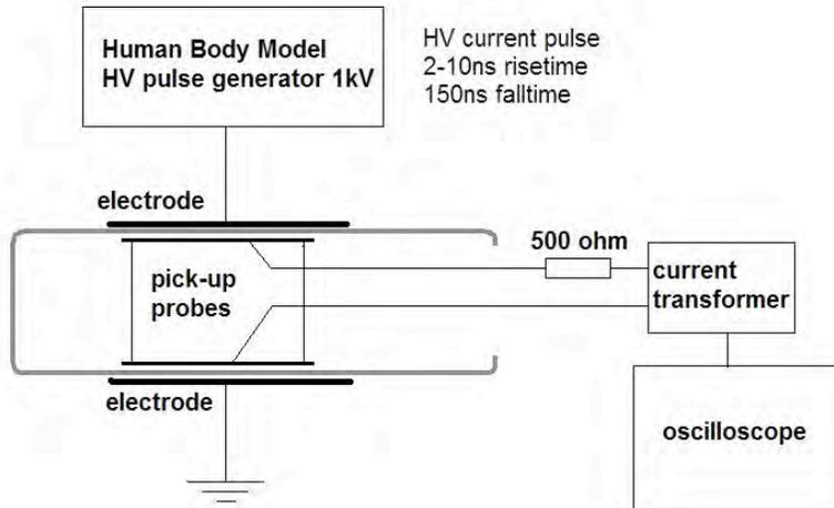
Figure 3.10 ESDA method for measurement of shielding performance
